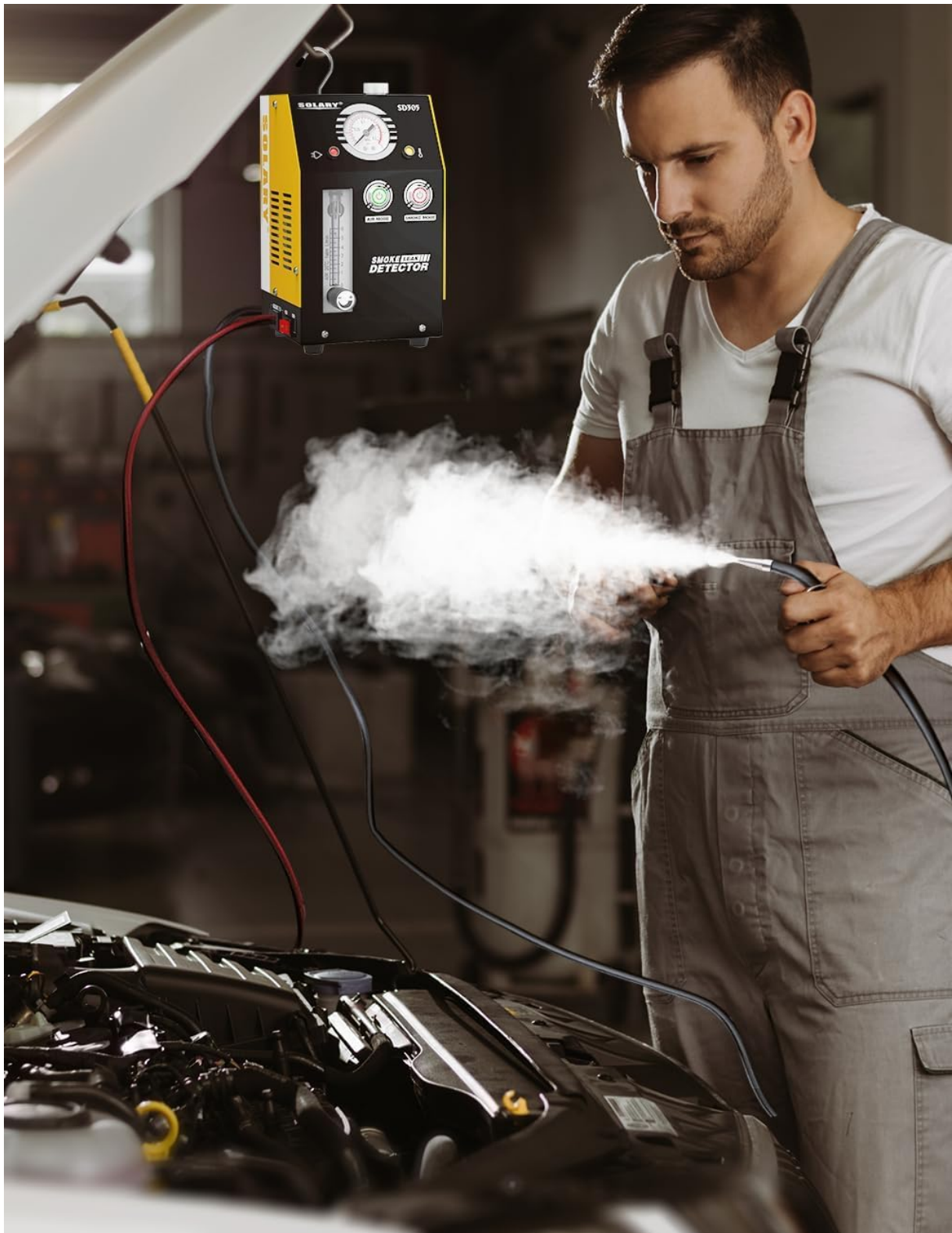
Image 6.3: A technician using the Solary SD305 to identify a leak in an automotive system.
