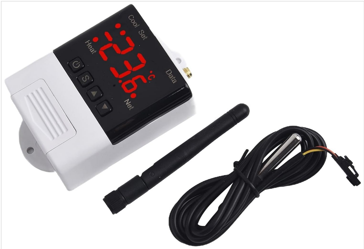
Image 1: Overview of the Hasaller DTC-2210 Temperature Controller, showing the main unit, detachable WiFi antenna, and the wired temperature sensor.
