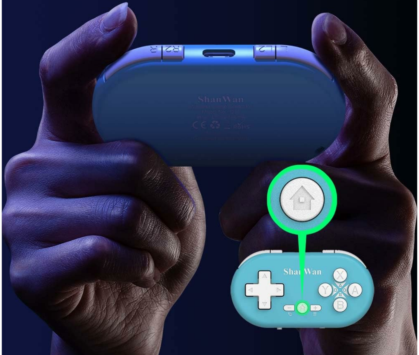
Figure 4.2: Visual guide for connecting the controller to a Nintendo Switch, showing menu navigation and the pairing button location.
