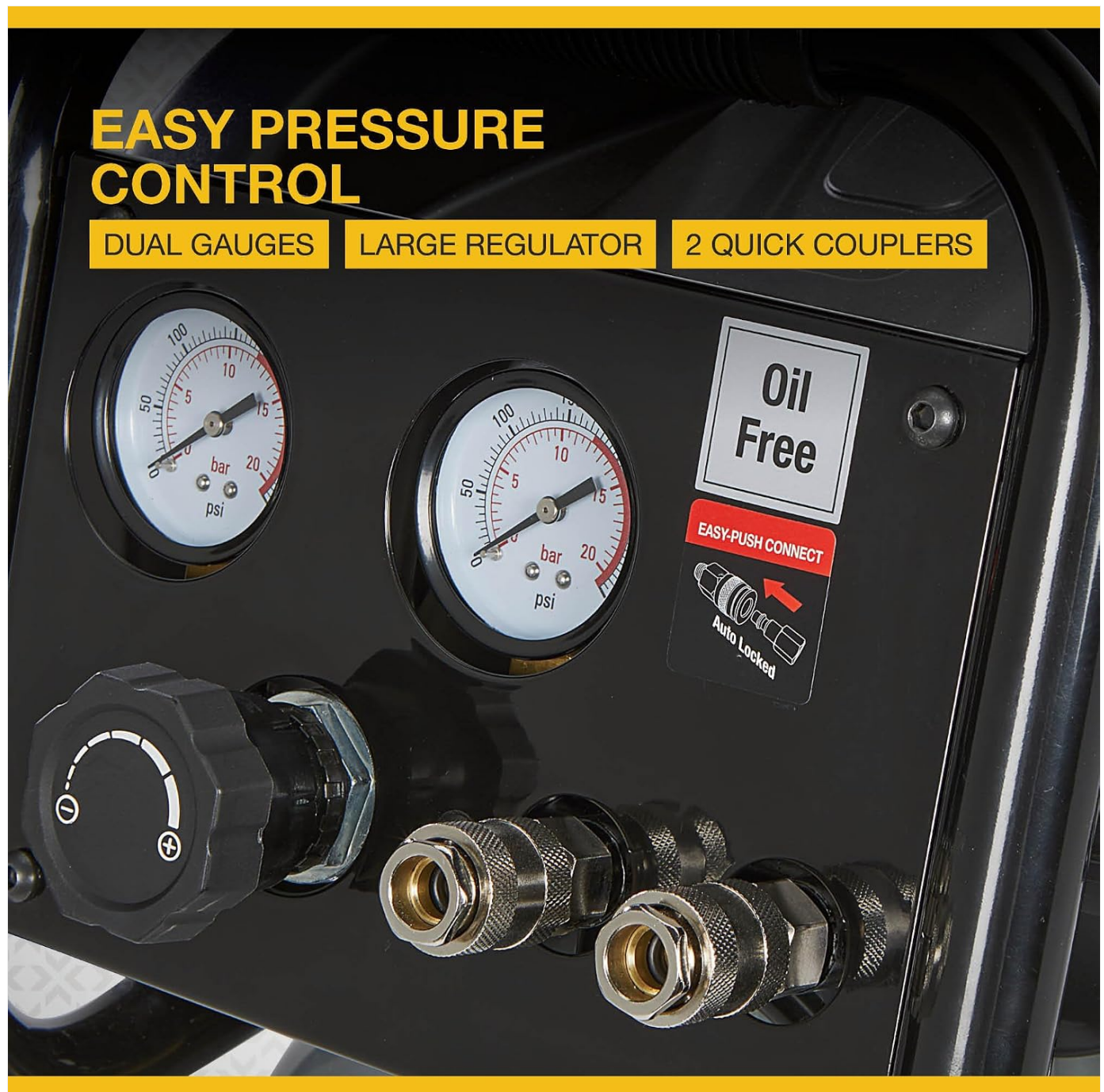
Figure 3.1: Control panel featuring dual gauges for monitoring tank and regulated pressure, a large regulator for pressure adjustment, and two quick couplers for tool connection.
