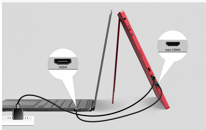
Image 4.2: Two-cable connection for devices without full-featured USB-C.
