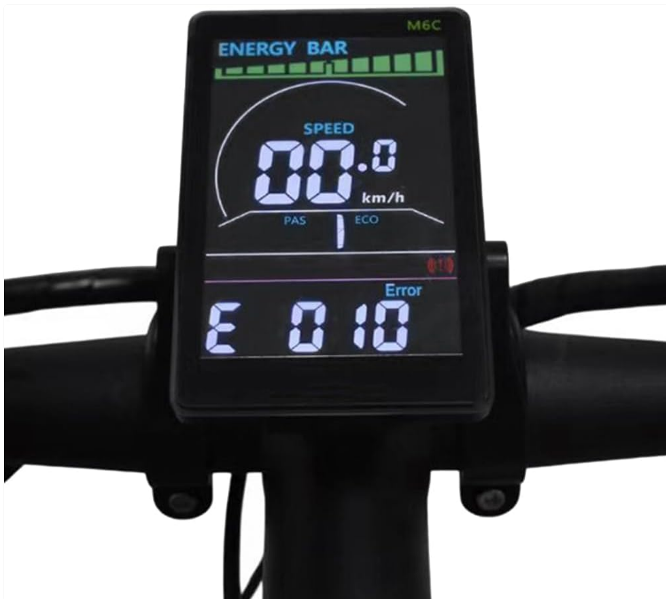
Figure 2: M6C Display Mounted on Handlebar. This image illustrates the M6C display as it would appear when mounted on an electric bike handlebar. The screen shows a speed of 00.0 km/h and an error code "E 010", indicating a potential issue.
