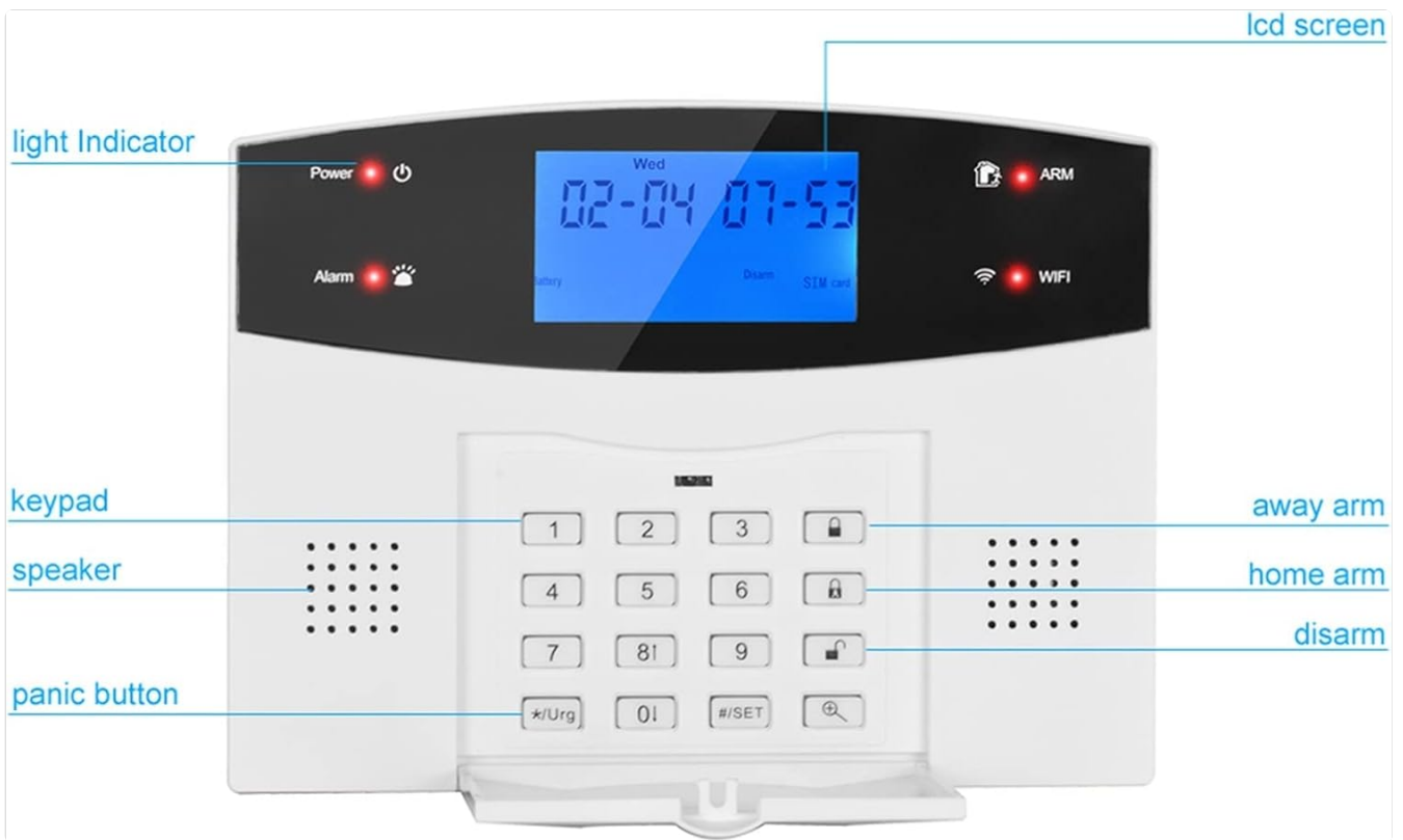
Figure 4: Main Control Panel Front View. A close-up of the JOXLOVER G2BW control panel's front, with labels pointing to key features: LCD screen, light indicator, keypad, speaker, panic button, and status indicators for power, alarm, battery, disarm, SIM card, ARM, and WiFi.
