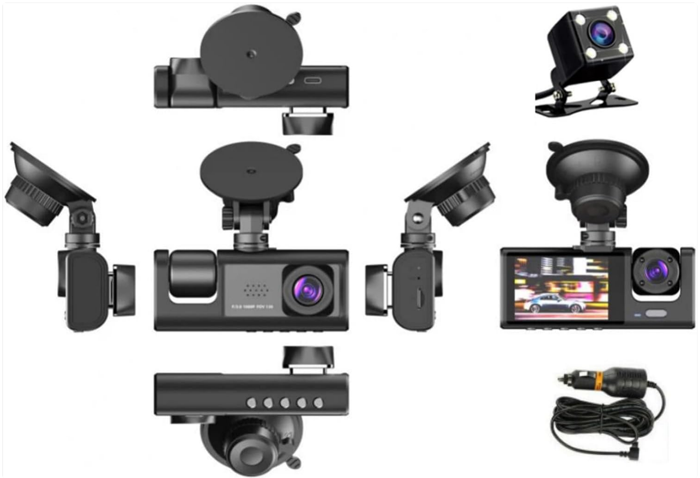
Image: Various perspectives of the Yoidesu Dash Cam, highlighting its compact form factor and the placement of its lenses, screen, and ports. The separate rear camera is also shown.
