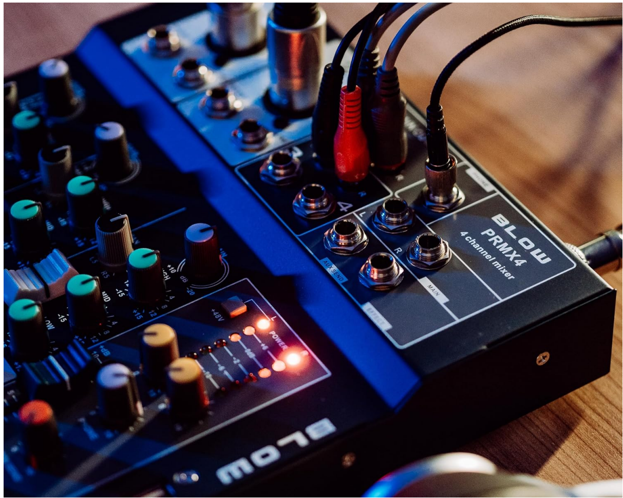
Figure 2.2: Close-up of the input and output connections. This image highlights the various ports for microphones, line inputs, main outputs, and auxiliary connections.
