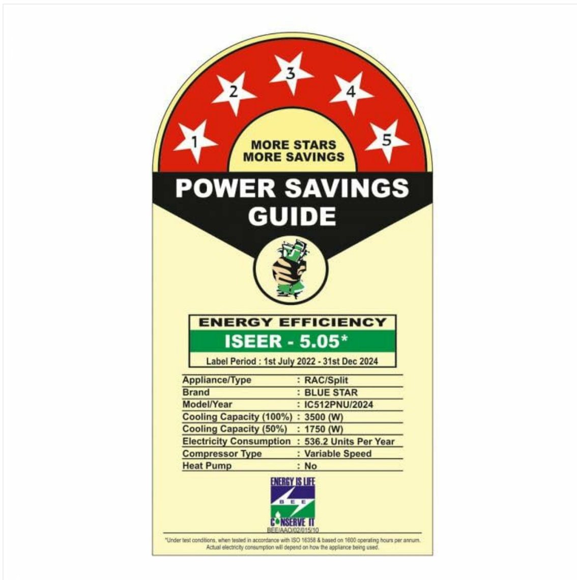
Figure 6: Power Savings Guide (Energy Efficiency Label) for the Blue Star IC512PNU. This label indicates a 5-star BEE rating with an ISEER of 5.05, detailing cooling capacity and electricity consumption.
