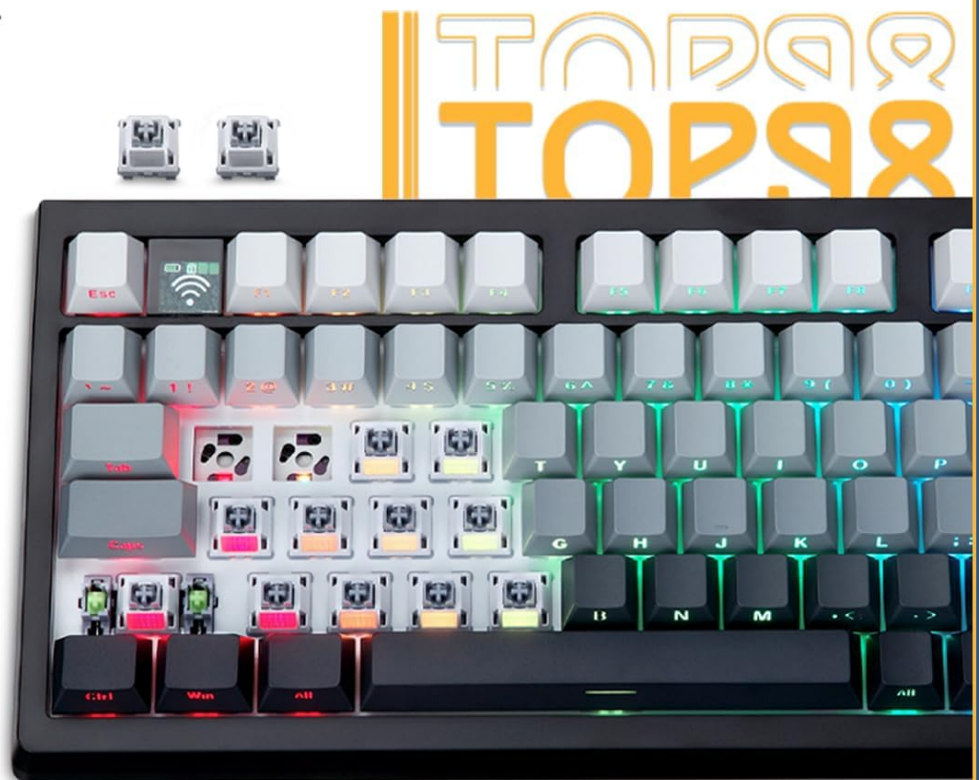
Figure 3.5: The keyboard features full hot-swappable switch sockets, allowing users to easily replace 3-pin or 5-pin mechanical switches to customize typing feel and sound without soldering.
