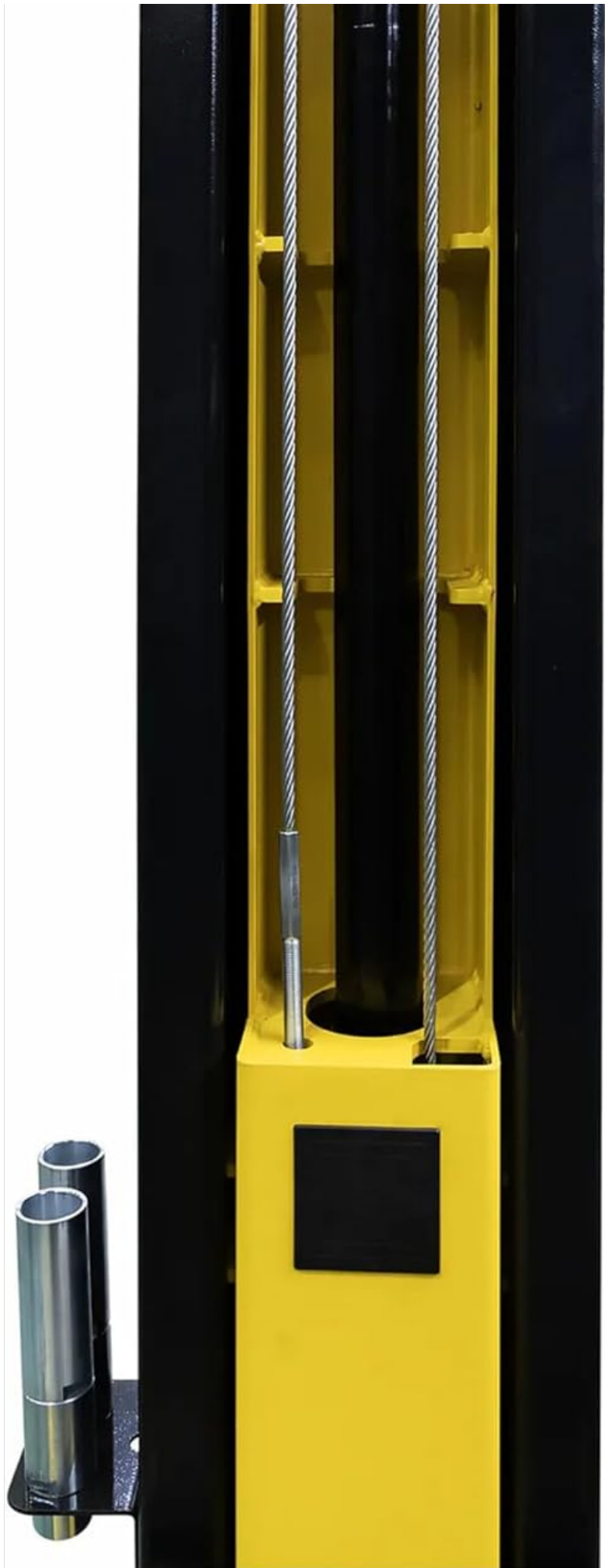
Figure 2.4: Detailed view of the hydraulic cylinder and equalization cables within the APlusLift AP-12SR lift column, essential for
