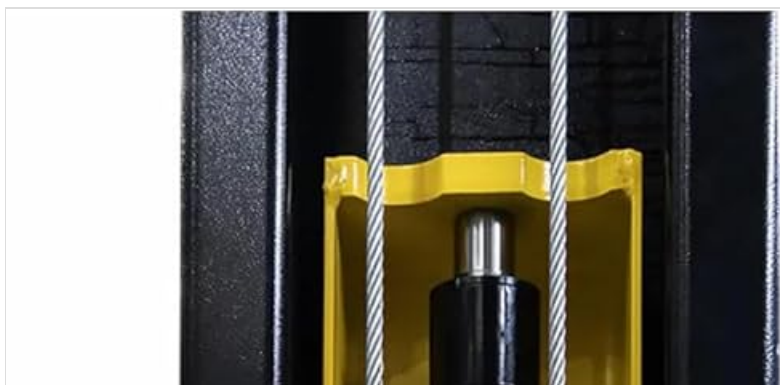
Figure 2.3: Close-up view of the top section of an APlusLift AP-12SR column, showing the cable routing and structural connection points.
