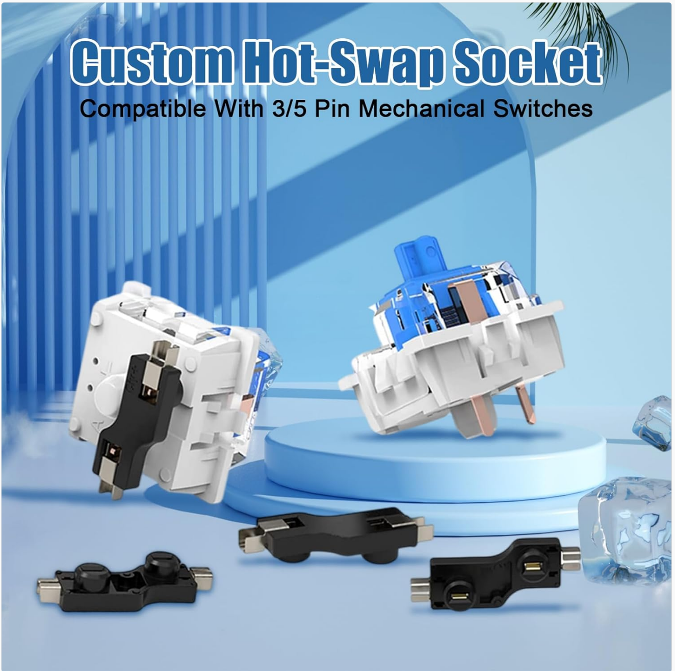
Figure 3.2: The CIY68's hot-swappable sockets are compatible with both 3-pin and 5-pin mechanical switches.
