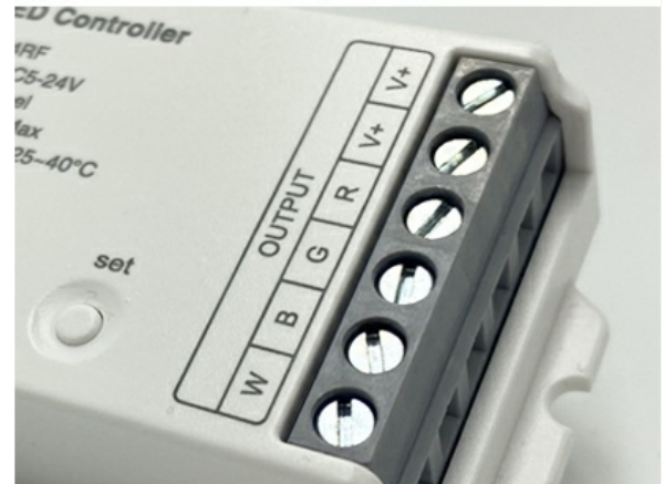
Image: Close-up view of the GIDEALED C04RF controller's DC power input and RGBW output screw terminals.
