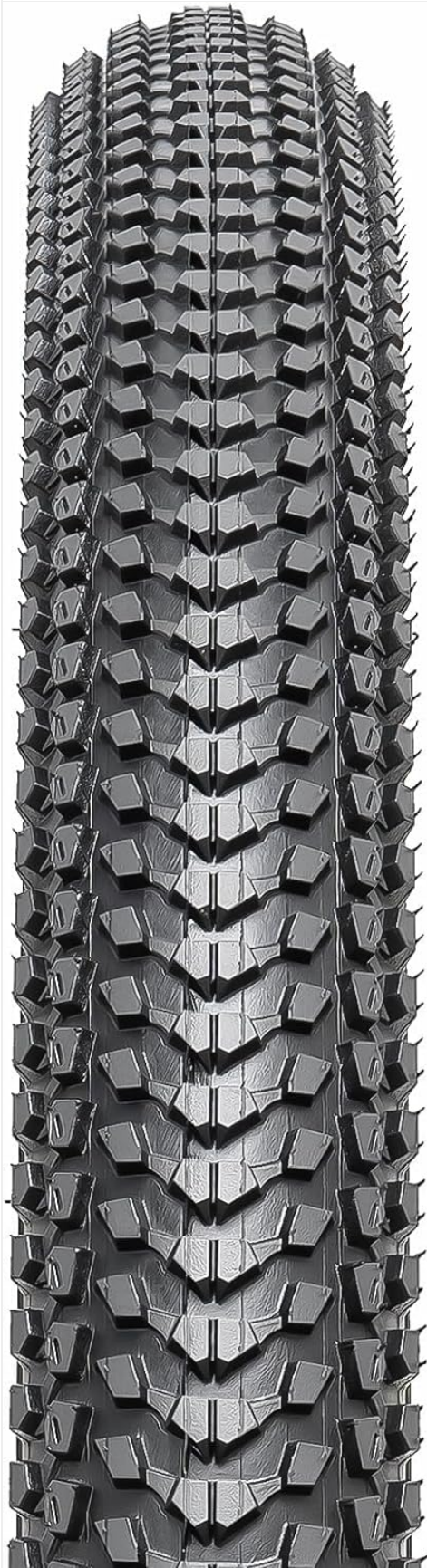
Image 1.2: Detailed view of the tire's high traction tread pattern, designed for increased friction and grip on various terrains.
