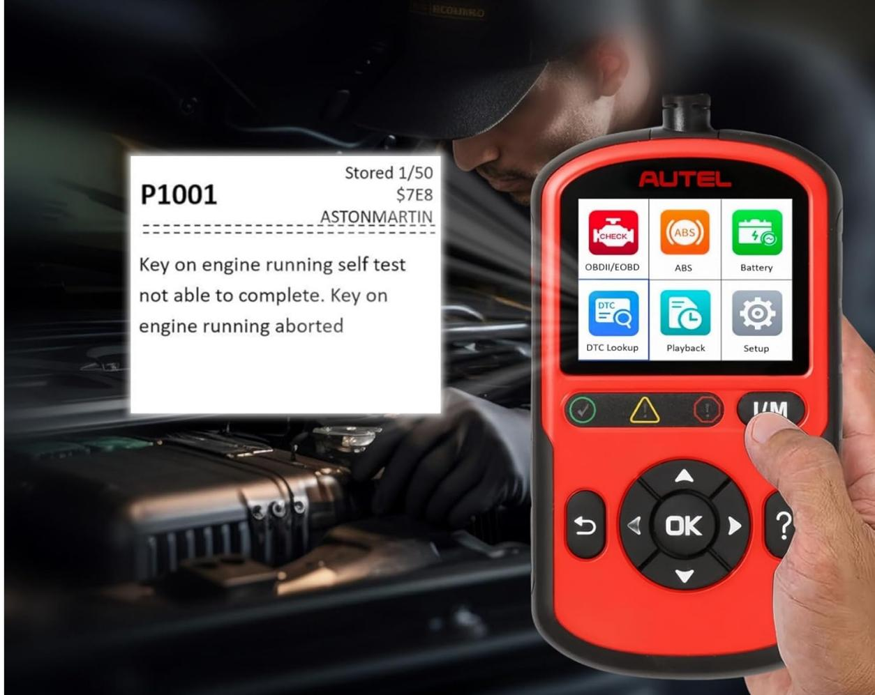
The image illustrates the DTC Lookup function of the Autel AL549. It shows the scanner displaying a diagnostic trouble code (P1001) along with its definition: 'Key on engine running self test not able to complete. Key on engine running aborted.' This feature helps users quickly understand the meaning of retrieved codes.
