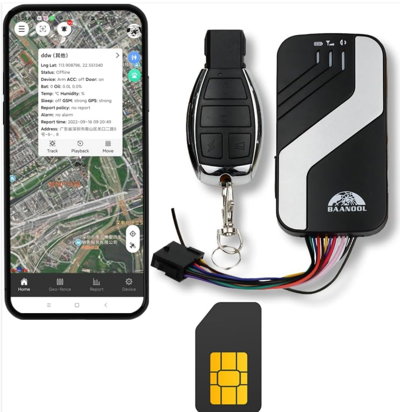
Image 2.1: The BAANOOL BN-403D GPS Tracker, showing the main unit, remote control, wiring harness, and SIM card.
