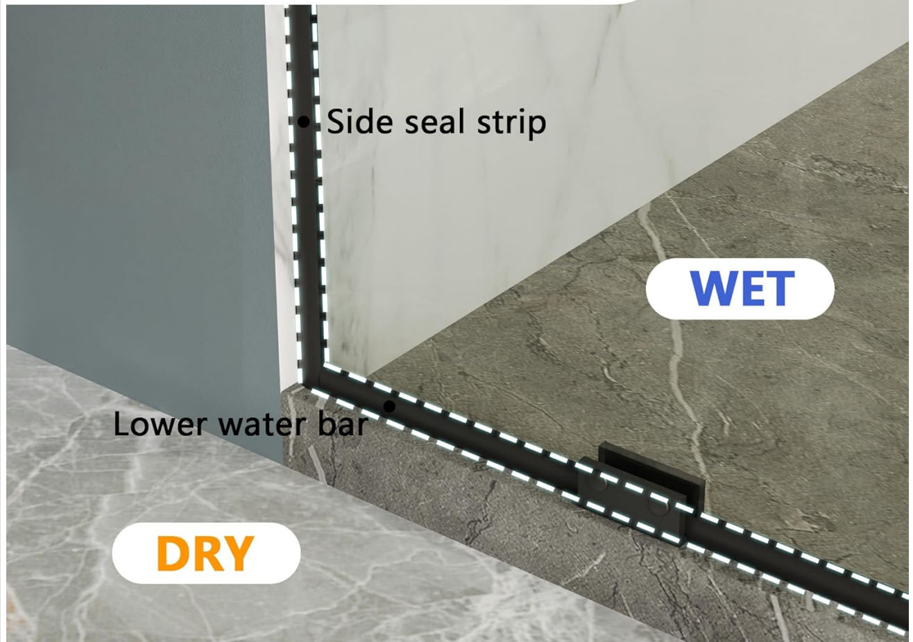
Image 6: Illustration of the waterproof design for wet/dry separation.
