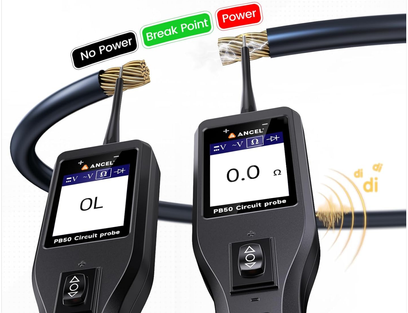
Figure 5.8: The AL-PB50 displaying "OL" for an open circuit and "0.0Ω" with a green LED for a short to ground, indicating a circuit break.
