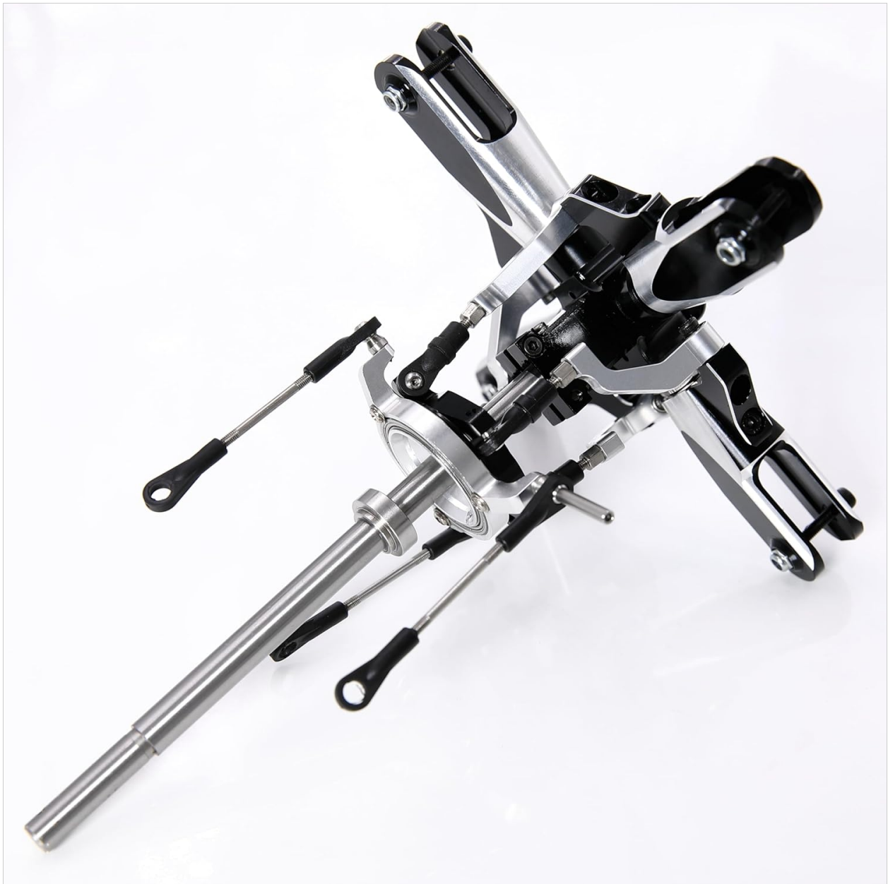
Figure 2: Detailed view of the rotor head assembly, showing the main shaft and control linkages.
