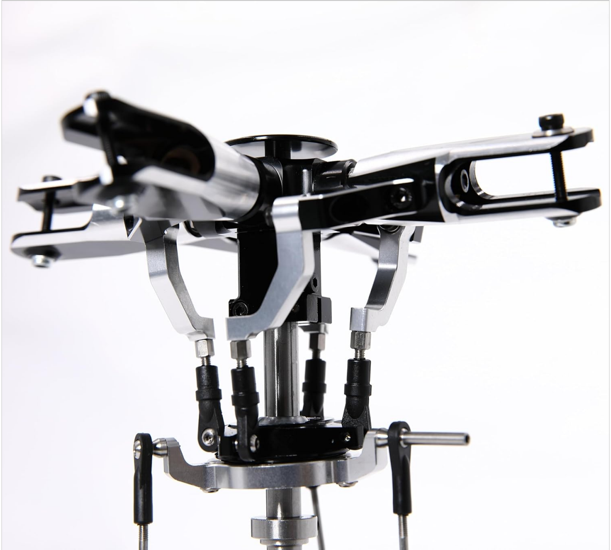
Figure 3: Close-up view of the Direct Flight Control (DFC) mechanism, highlighting the linkage points.
