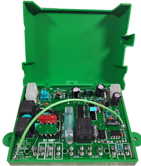
Image: The Aeipiraza Micro P-711 circuit board housed within its protective green casing, showing the internal components and connectors.
