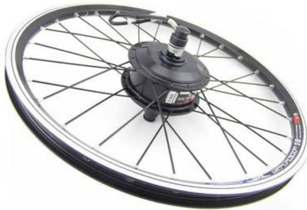
Image 4.3: The AKM-36V250W hub motor integrated into a 20-inch bicycle wheel.
