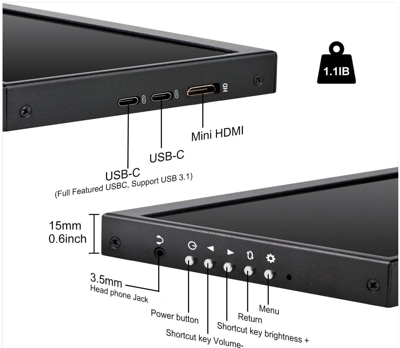
Figure 3.2: Detailed view of the monitor's side, showing the Mini HDMI port, two USB-C ports (one full-featured), a 3.5mm headphone jack, power button, menu button, and shortcut keys for brightness and return functions.
