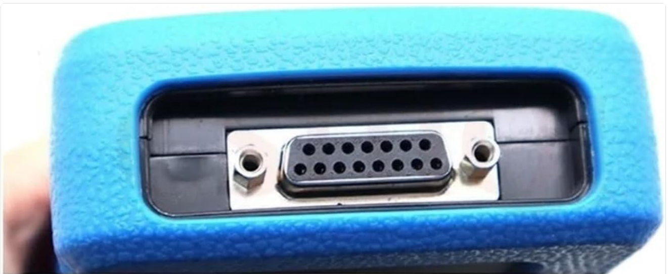
Figure 2.2: A close-up view of the multi-pin connector port on the XTP-SP820 device, typically used for connecting the OBD-II cable or other accessories.
