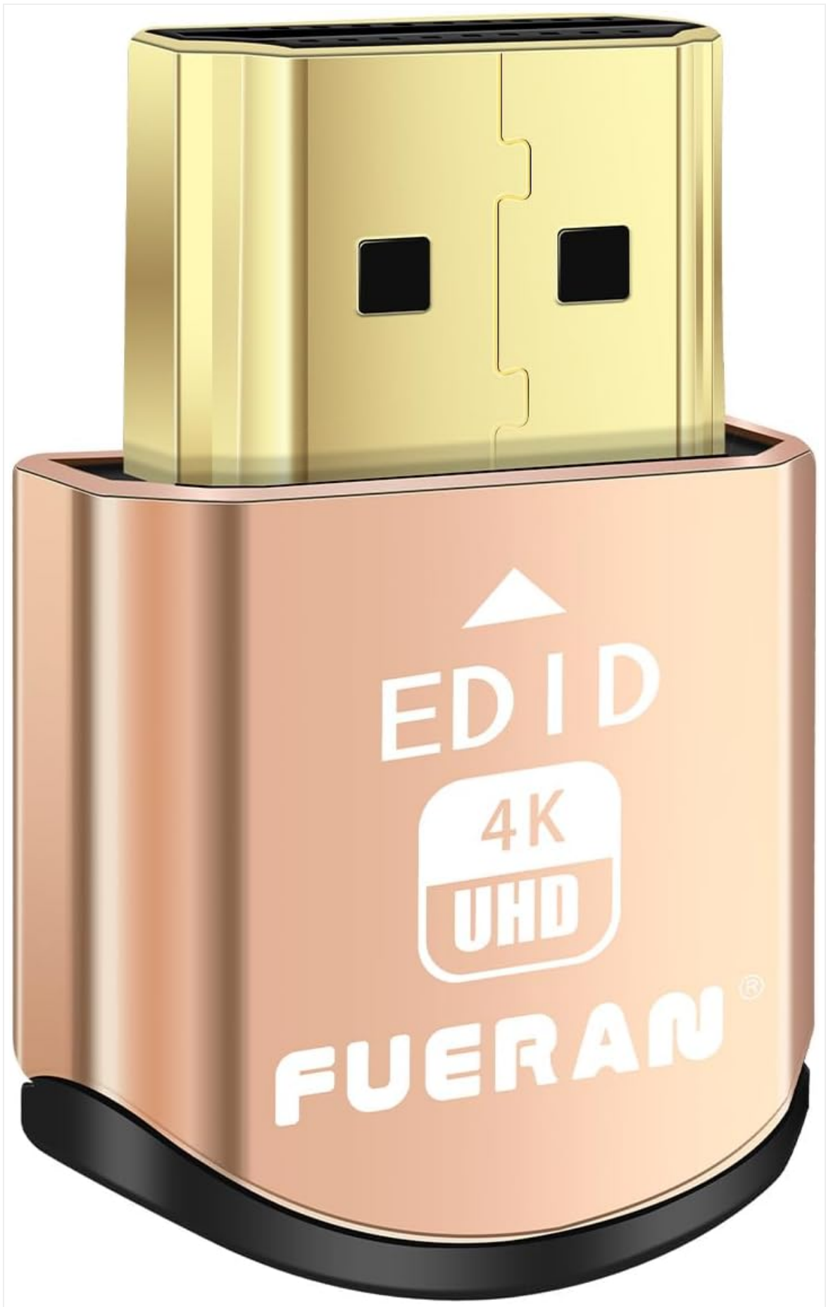
Image 1.1: The FUERAN 4K-1P HDMI Dummy Plug, a compact device designed to emulate a display.
