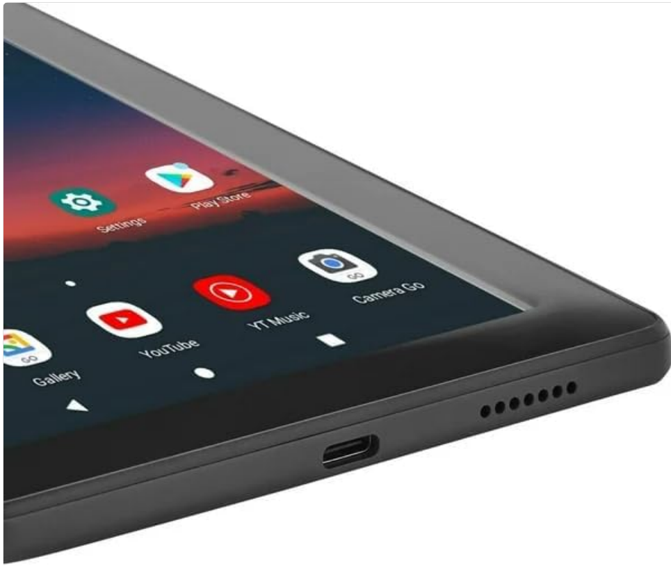
Figure 1: USB-C charging port and speaker grille.
