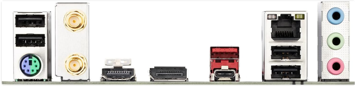
Figure 3.3: Rear I/O panel showing various ports including USB, Wi-Fi antenna connectors, HDMI, DisplayPort, USB 3.2 Gen 2x2 Type-C, Ethernet, and audio jacks.
