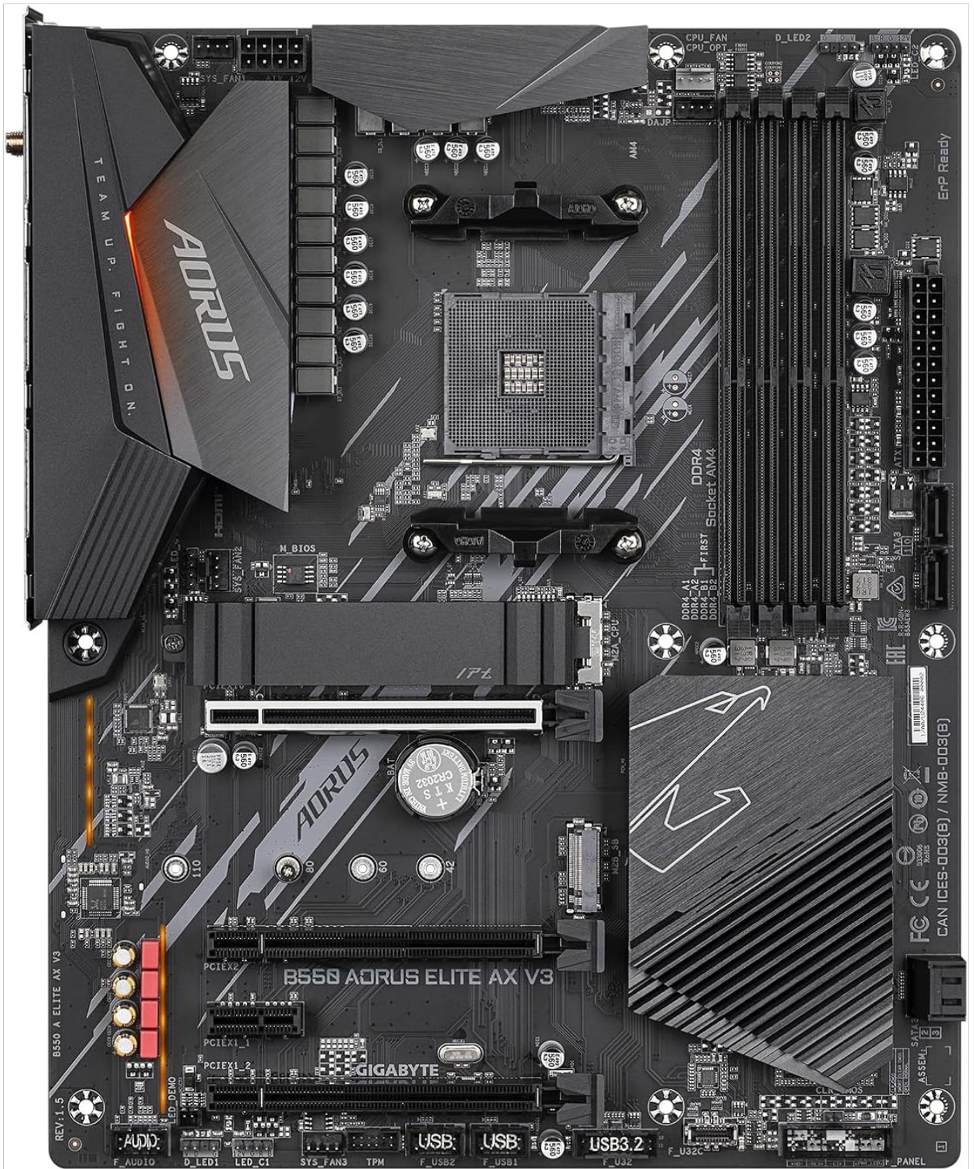
Image 2.1: Top-down view of the motherboard, showcasing component layout and heatsinks.
