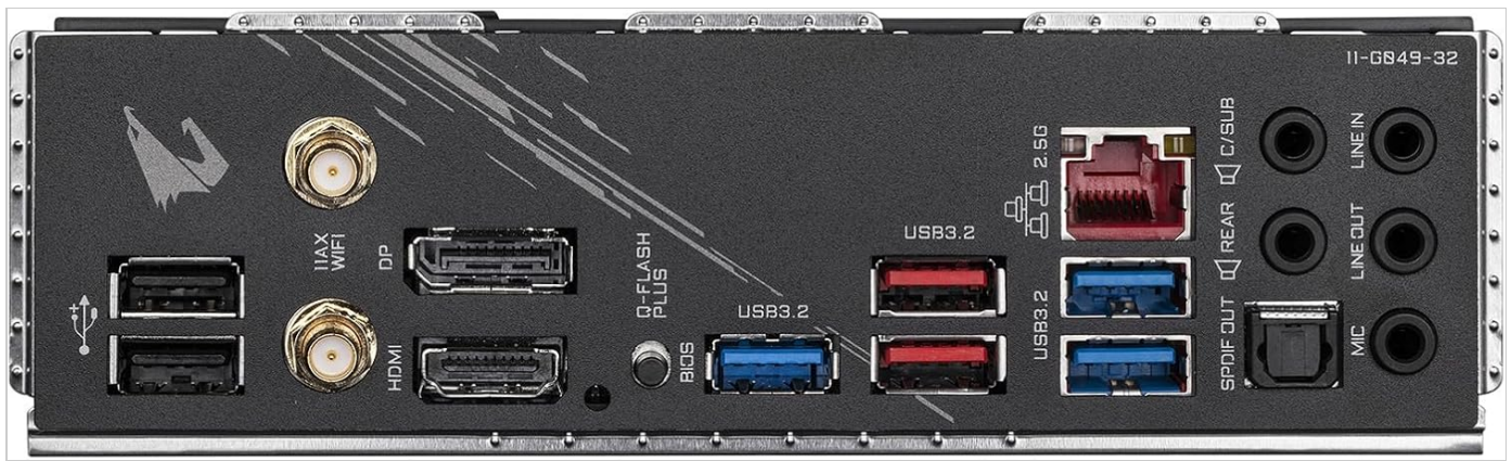
Image 3.2: Rear I/O panel, highlighting the Q-Flash Plus button and dedicated USB port for BIOS updates.
