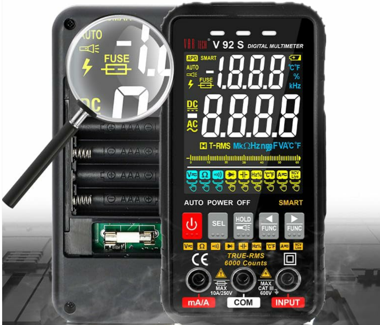
Figure 7.1: The intelligent anti-burn function prompt, indicating the location of the fuse for replacement.
