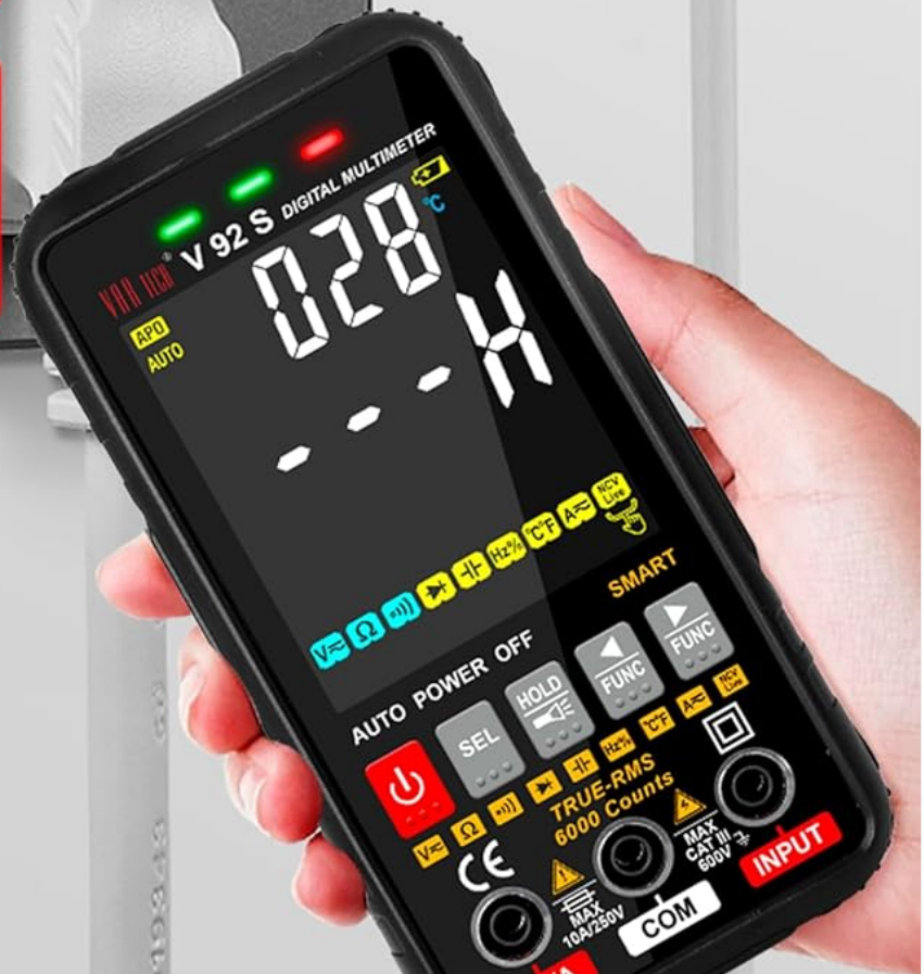
Figure 6.2: Auditory and visual alarm during NCV (Non-Contact Voltage) testing, indicating the presence of AC voltage.
