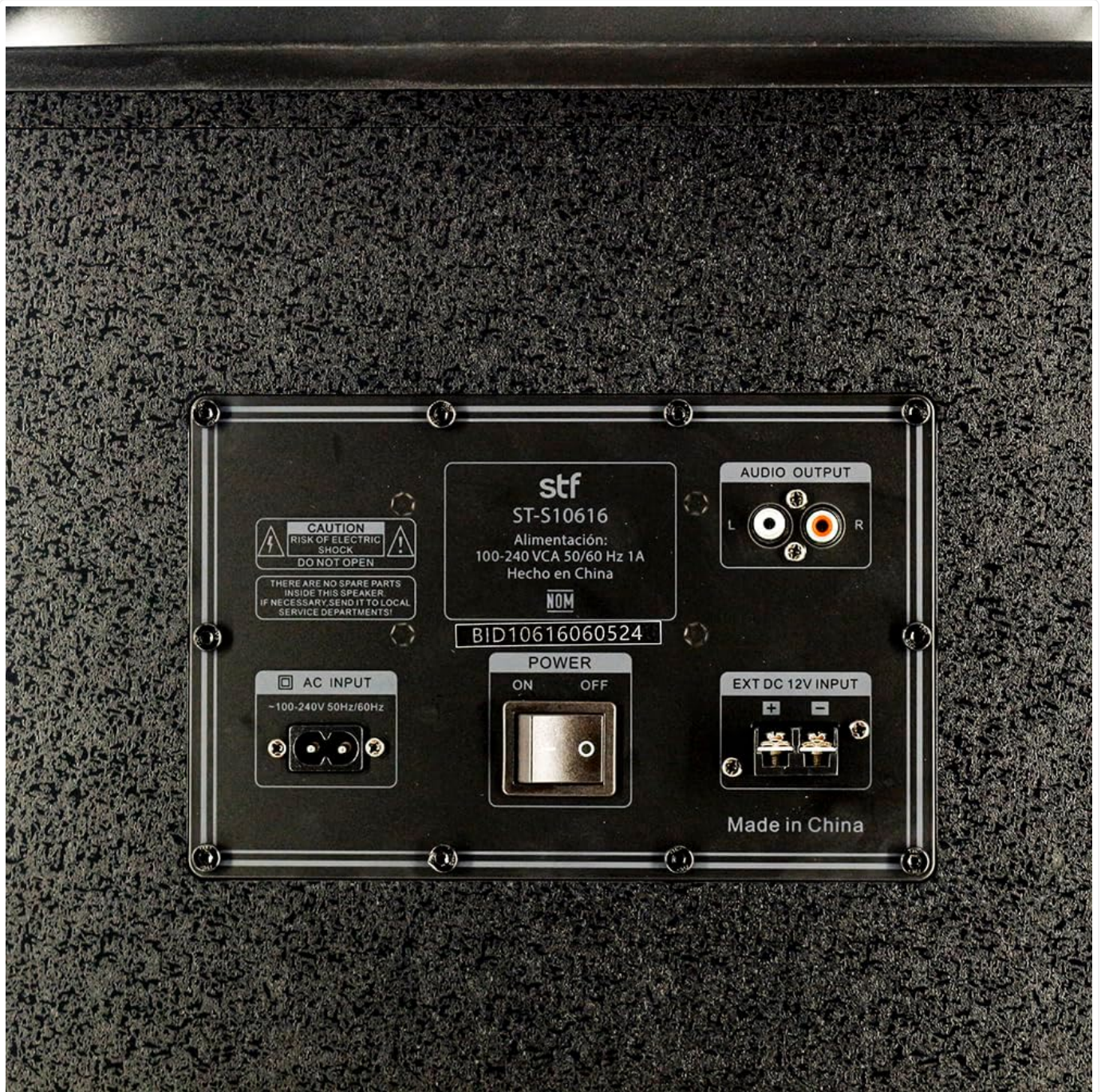
Figure 4: Rear panel with AC power input, external DC 12V input, power switch, and audio output.
