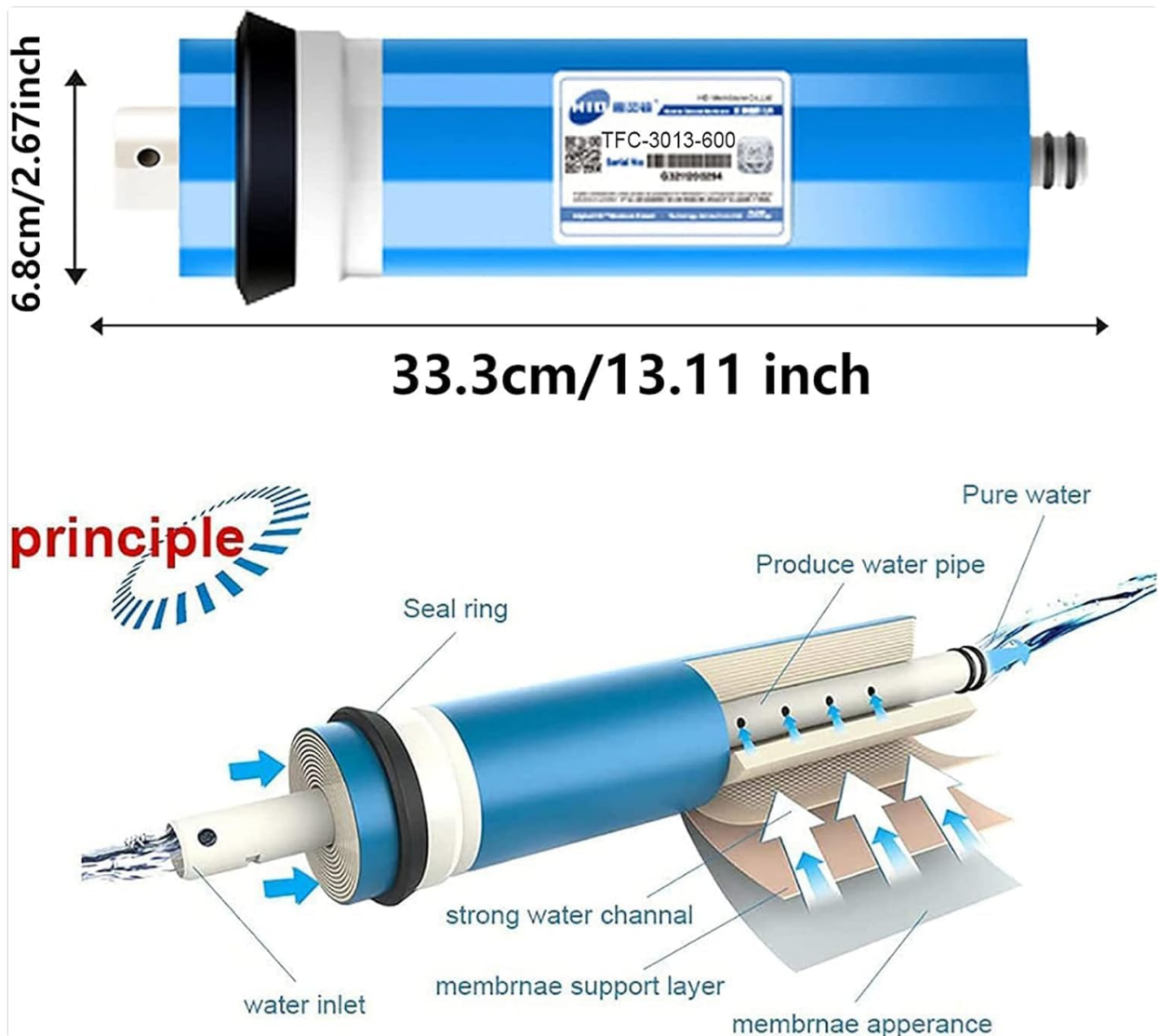
Image 3.1: Dimensions of the 3013-600 GPD RO Membrane Filter.
