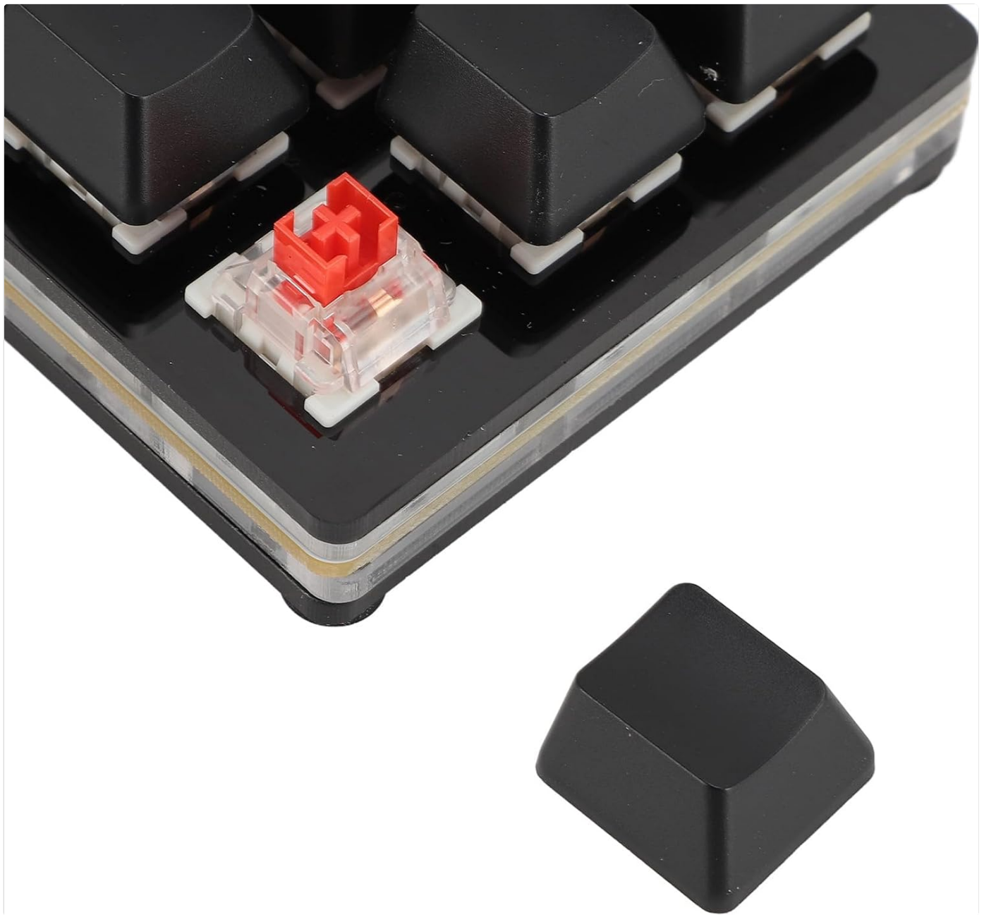
Image 5.2: A close-up view of a red mechanical switch with a keycap removed, demonstrating the hot-swappable design.
