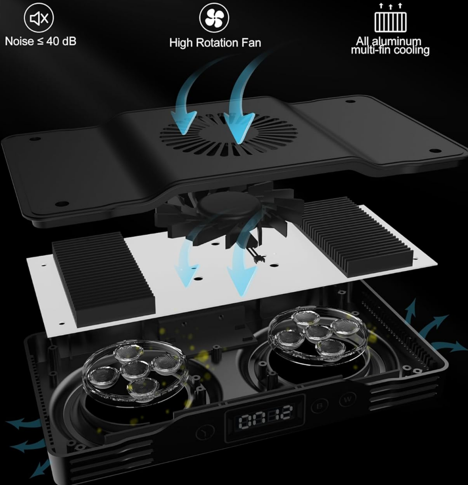
Figure 4: Exploded view of the A036's heat dissipation components.
