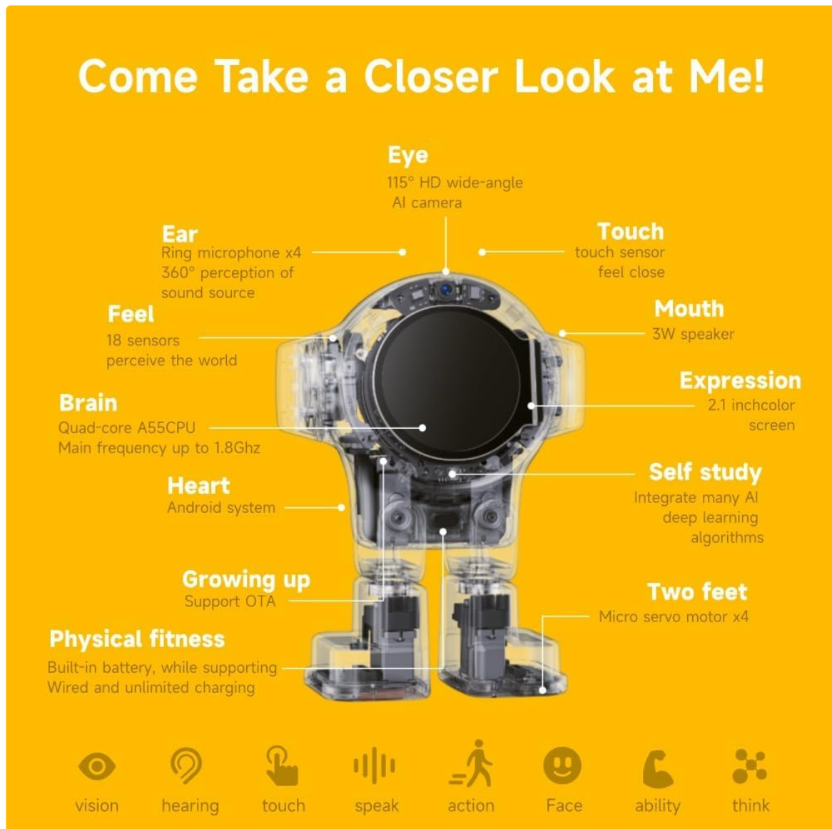
Image: An exploded view of the Rux robot highlighting its internal components such as the quad-core A55 CPU, Android system, 18 sensors, 5MP camera, microphones, speaker, and micro servo motors.
