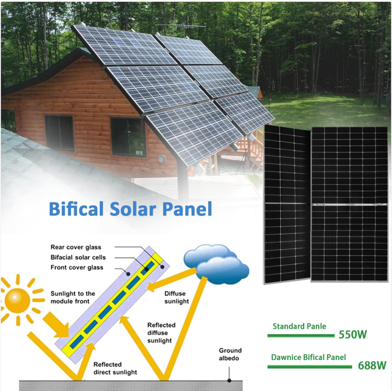
Figure 4.1: Bifacial Solar Panel operation principle.
