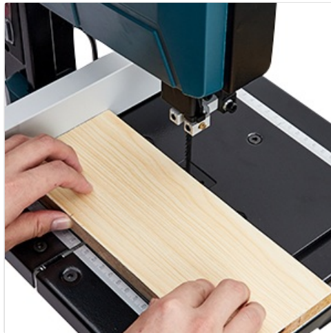
Figure 5.1: Demonstrates cutting a straight line using the bandsaw, typically guided by the rip fence.
