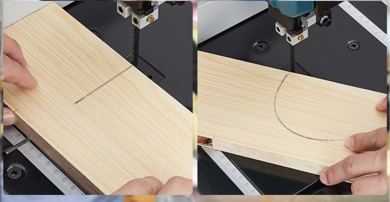
Figure 5.2: Illustrates the versatility of the bandsaw for both straight and curved cuts, allowing for intricate designs.
