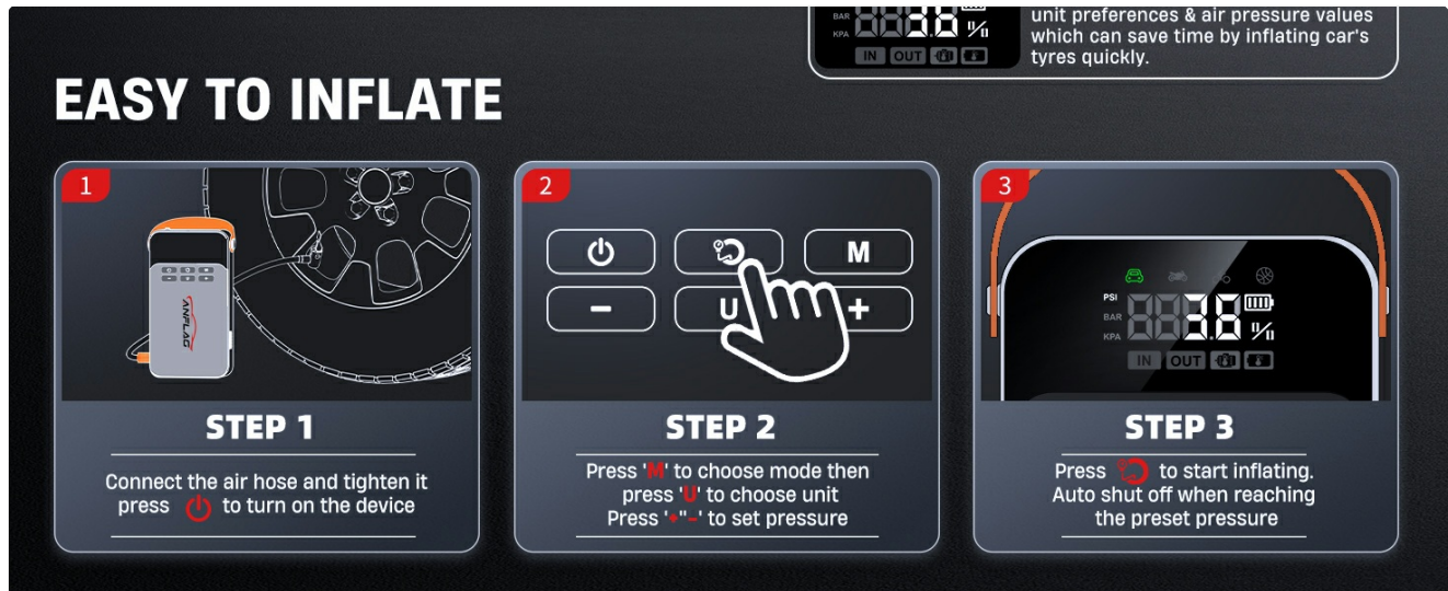
Figure 6.3: A three-step visual guide on how to easily inflate tires using the ANFLAG BD50's integrated air compressor.
