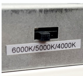
Image: A close-up of the CCT slider switch on the light panel, alongside three images showing the light output at 4000K (Cool White), 5000K (Daylight), and 6000K (Daylight Deluxe), demonstrating the selectable color temperature feature.
