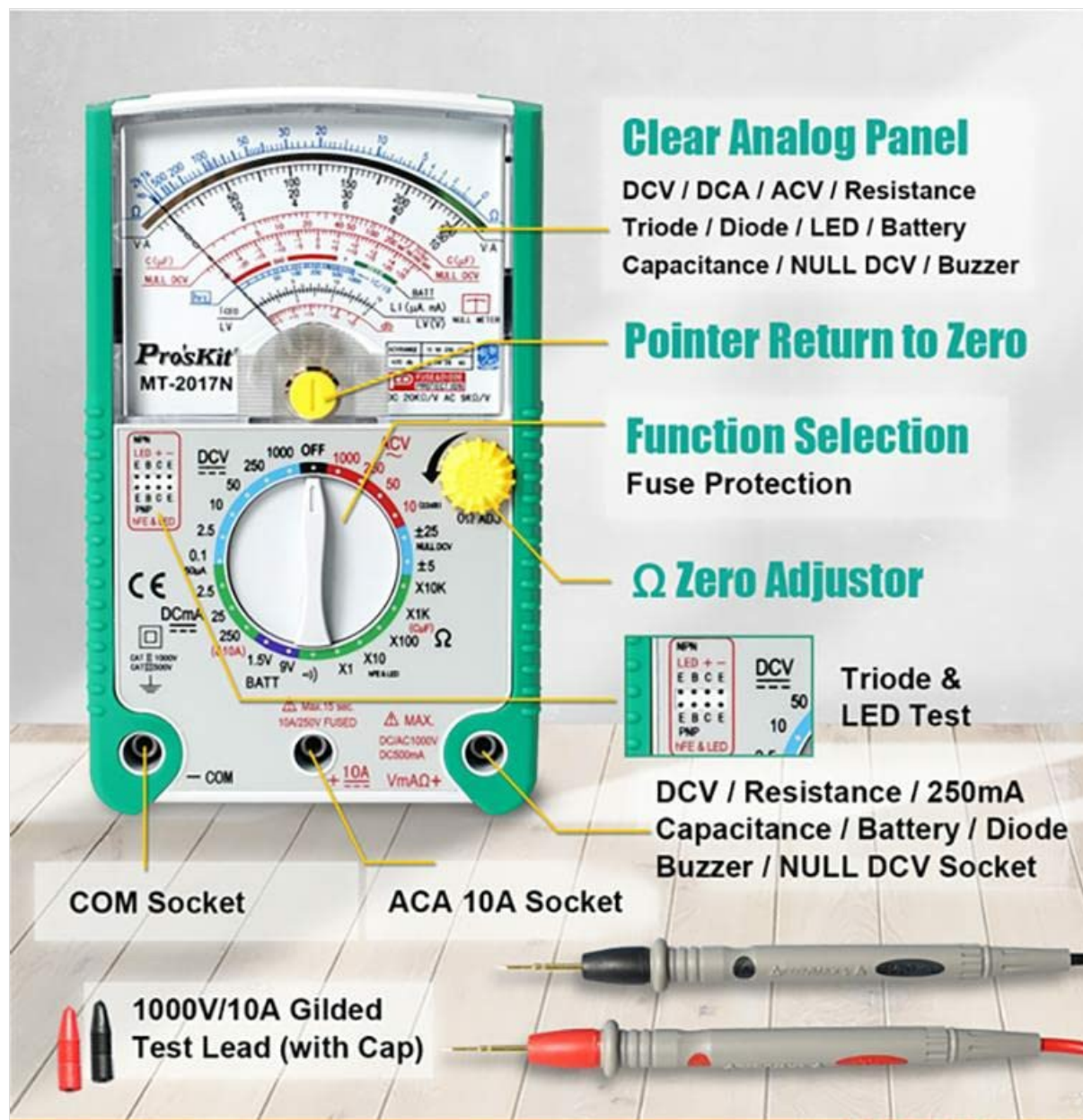
Figure 2.2: Detailed view of the multimeter's analog panel, showing the pointer, function selection dial, zero adjustor, COM socket, ACA 10A socket, and test lead connections.
