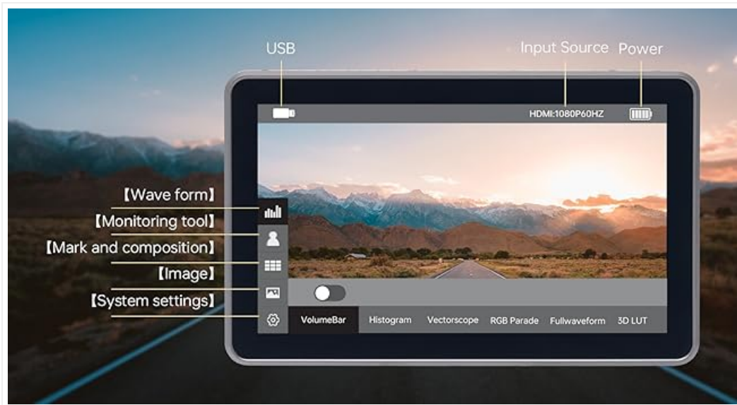
Figure 3.2: Overview of the DC-X3's touchscreen interface, showing menu options and touch gestures.
