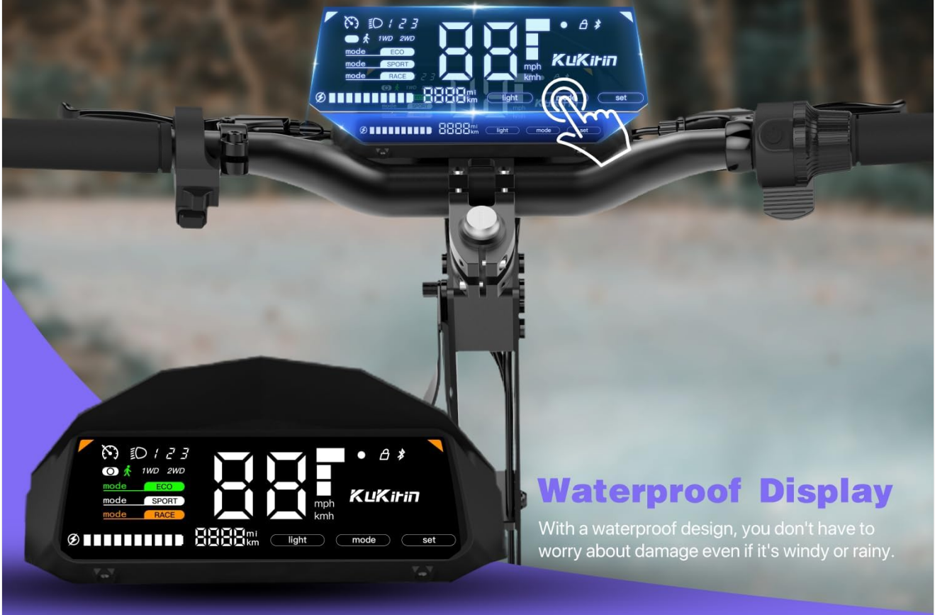
Image: Close-up of the Kukirin G4's waterproof Touch LED display, showing speed, speed mode, battery power, lighting status, and cruise control indicators.
