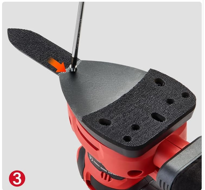
Figure 3: Step-by-step guide showing how to change the sanding pads. (1) Unscrew the existing pad. (2) Attach the desired sandpaper to the new pad using the hook and loop system. (3) Secure the new pad to the sander with screws.
