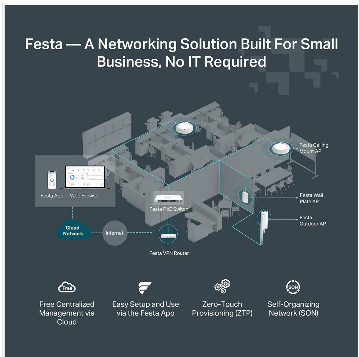
Figure 5: Diagram illustrating a Festa networking solution for small businesses, showing the integration of the VPN router, PoE switch, and various access points (ceiling mount, wall plate, outdoor) managed via the Cloud Network.
