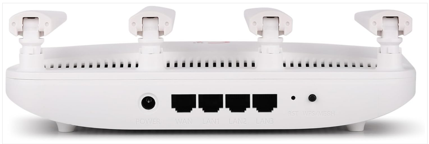
Image 3.2: The rear panel of the OLAX Scorpio Giga Home AX1800 Router, displaying the power input, one WAN port, three LAN ports, and a combined Reset/WPS/Mesh button.
