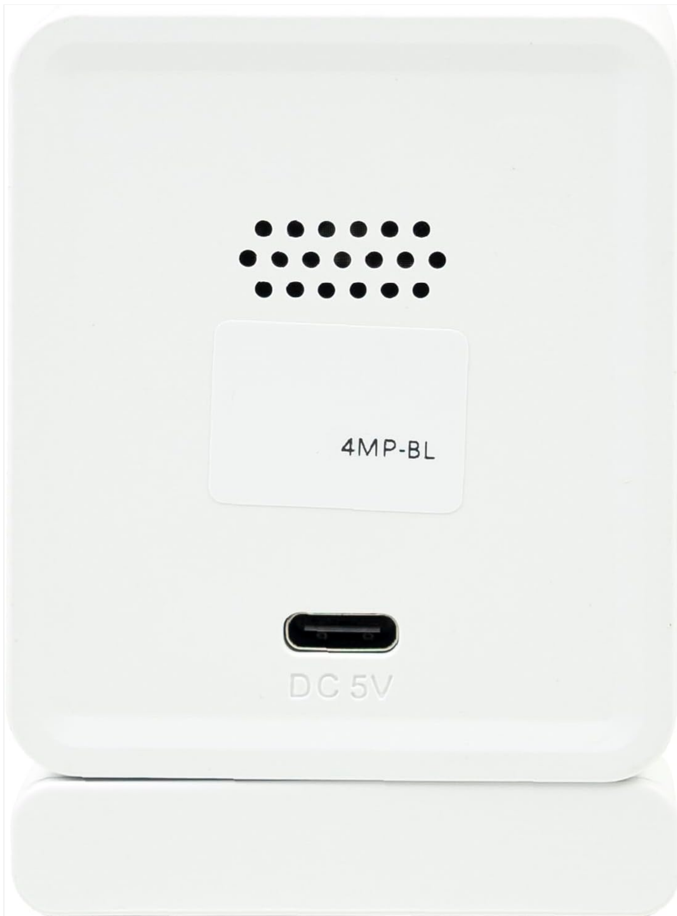
Image 3.2: Rear view of the PNI IP744 camera, showing the DC 5V power input port.
