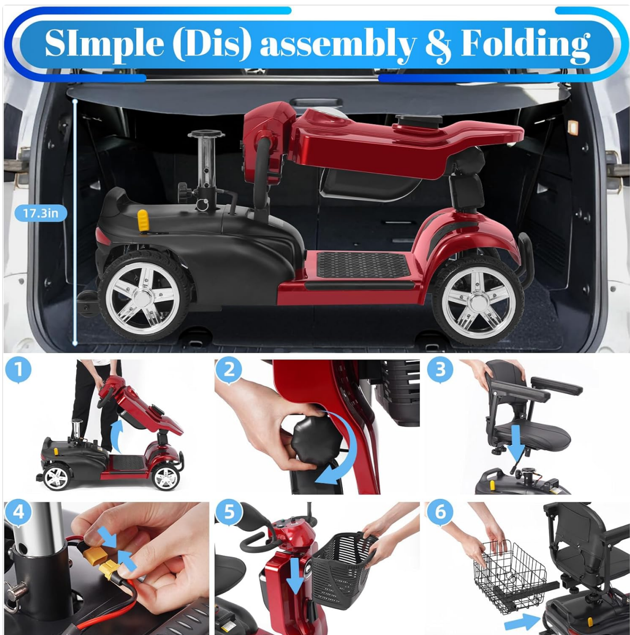
Image: Step-by-step visual guide demonstrating the simple assembly and folding process of the Ecomobi MS02 Pro, including how it fits into a car trunk.
