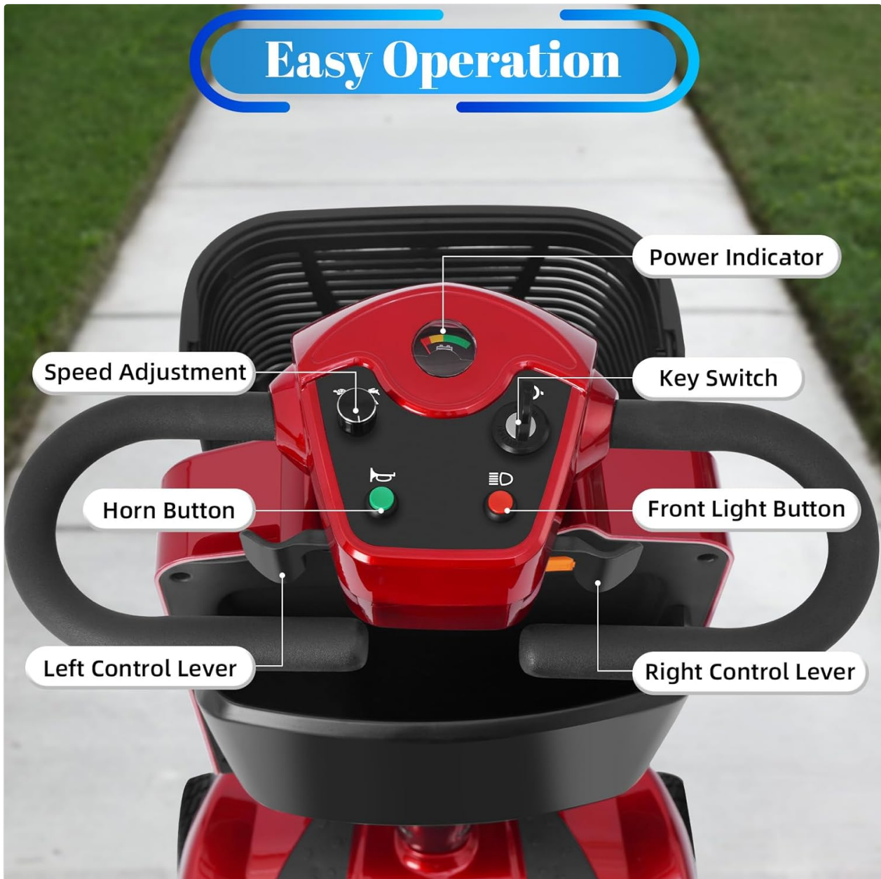
Image: Close-up view of the scooter's control panel, labeling the power indicator, speed adjustment, key switch, horn button, front light button, and left/right control levers.
