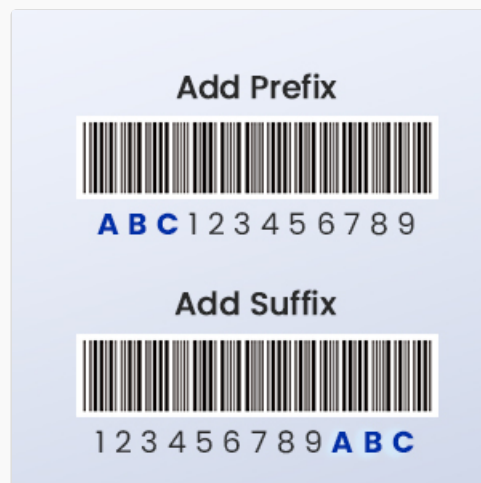
Image 6.2: Add Prefix/Suffix. This image demonstrates how custom characters, such as 'ABC', can be appended as a prefix before or a suffix after the numerical data of a scanned barcode.
