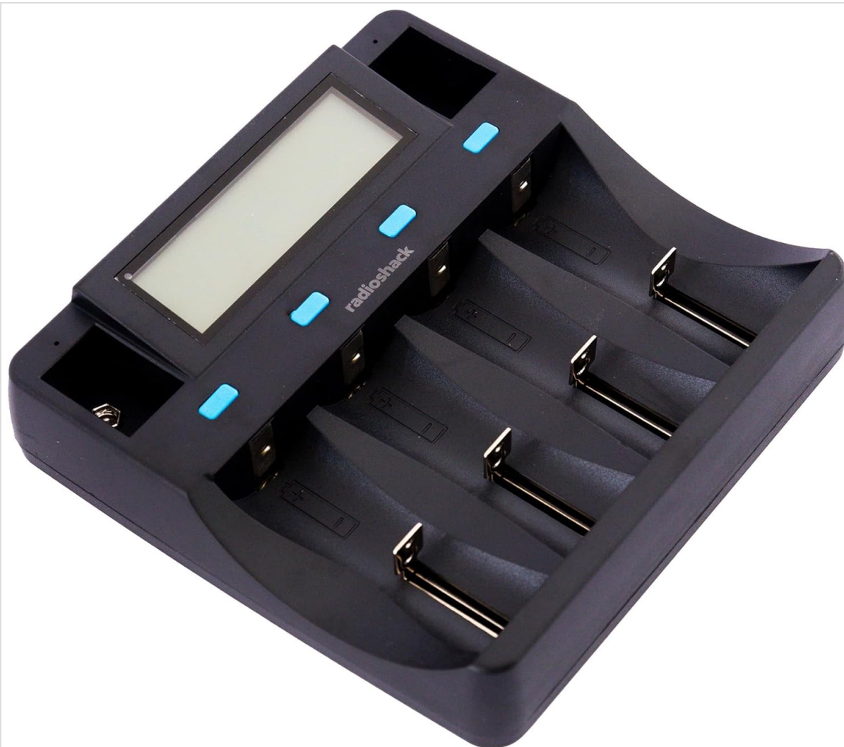
Image: Top-down view of the charger, showing the digital display and four main charging bays, plus two 9V slots.
