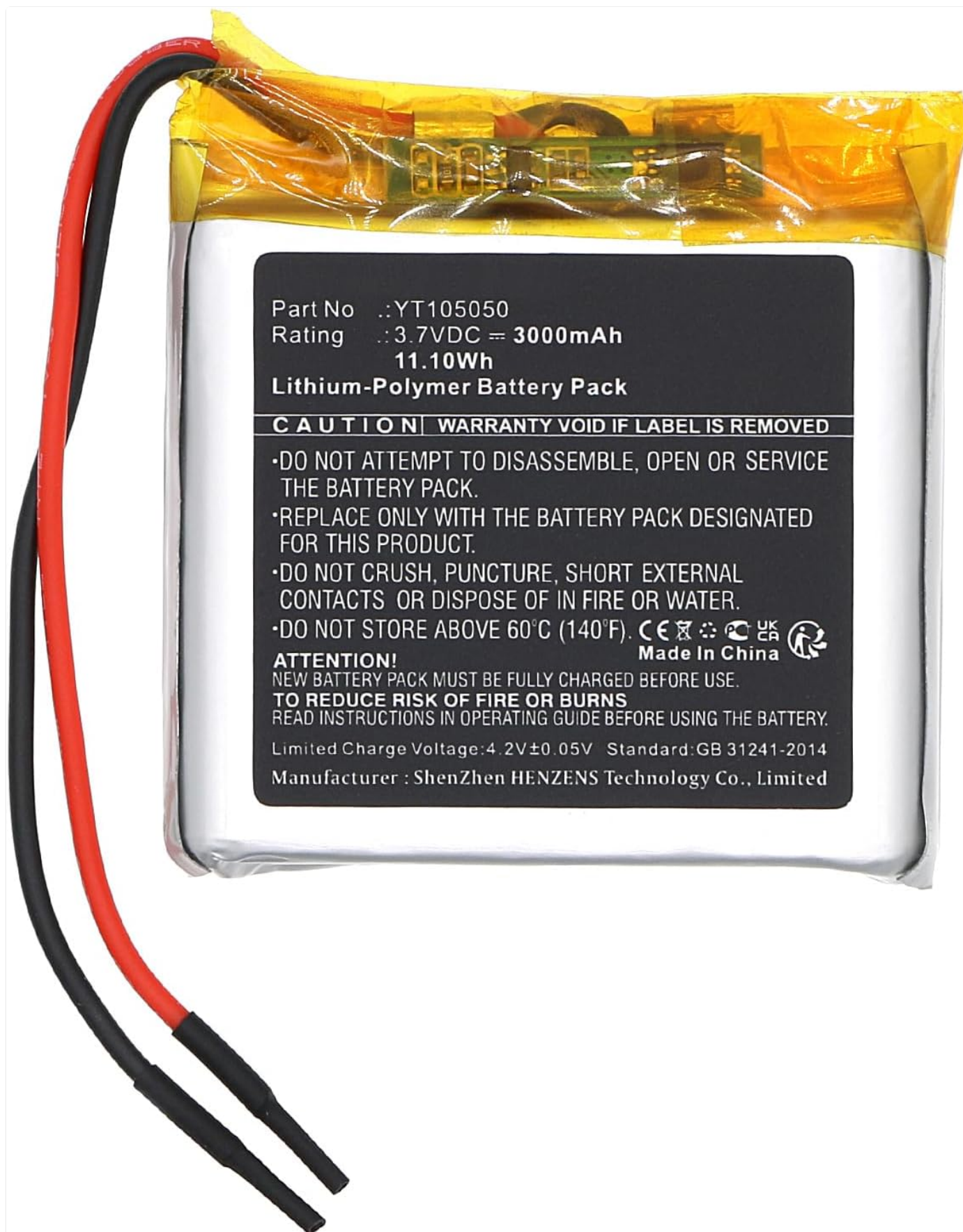
Image 1.2: Bottom view of the Synergy Digital YT105050 battery, highlighting important safety warnings and manufacturer information.
