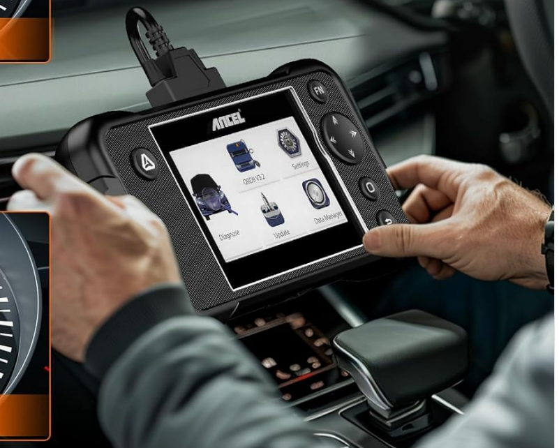
Figure 4.2: ANCEL FX3000 Elite Reading and Clearing Fault Codes.
